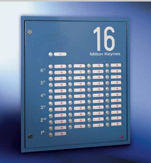
Fig. 32/1 Bespoke bell and intercom box with 20 mm aluminium plaster frame and RSA for flush fitting, with drop down front.
