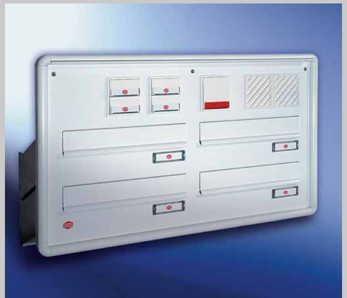
Fig. 25/4 Box format 300 x 110 x 265 - 410 mm, hinged steel front plate with RS1001 radius-profile closing frame. Letter plates 265 x 33 mm.
