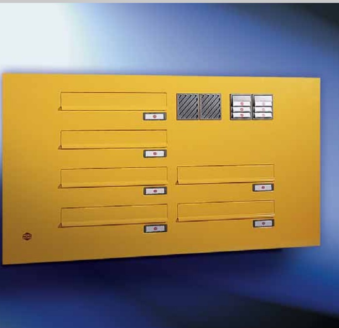
Fig. 22/3 Box format 370 x 110 x 270 mm, 24 mm steel front plate, with thermal break for mounting in door profile. Letter plates 335 x 33 mm.
