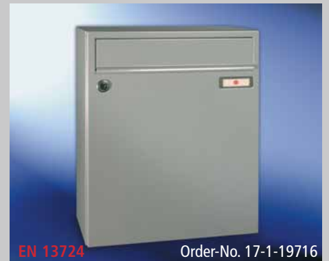
Fig. 36/6 Mail box 370 x 440 x 145 mm, with letter plate 335 x 33 mm. With RS50 2-point-locking. (*these models can also be supplied in V4A stainless steel).
