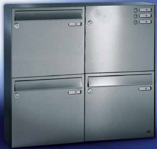
Fig. 12/4 Box format 370 x 330 x 100 mm, with RSA , and V4A stainless steel sheet casing. Letter plates 335 x 33 mm.
