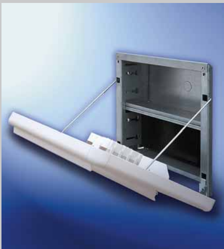
Fig. 26/1 Box format 260 x 110 x 265 - 410 mm, hinged aluminium front plate, with RSA and RS1001 aluminium radius-profile closing frame. Letter plates 230 x 33 mm.
